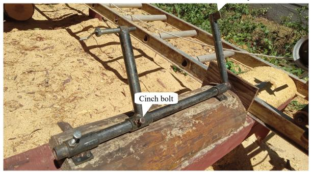
I have been using these log holders on my mill for three seasons. They are simple to build and easy to use. Before making the brackets I was slabbing smaller logs, as the logs got bigger I needed a way to position the larger logs for my 18" bar. I am also able to hold the logs to make finished boards.
